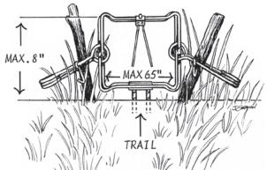
bait, lure, or attractant must be no greater than 6.5 inches inside the jaw hinges (160s) and only may be set such that no part of the body-gripping surface is more than 8 inches above the ground (see figure above).
